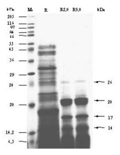
Figure 3. SDS-PAGE electrophoresis of pea protein extract and its trypsin hydrolysates (DH 2.0 and 5.0). Mw - markers, R –pea protein extract, R 2.0 and R 5.0 - trypsin hydrolysates with DH 2.0 and 5.0
